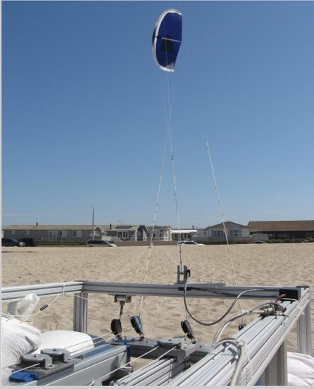
Fig. 1. Example of small-scale prototype built at the University of California, Santa Barbara, employing a curved flexible kite.
