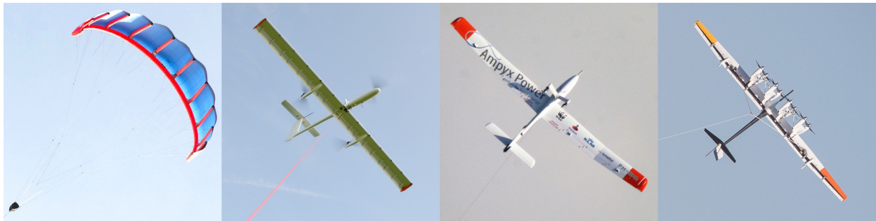
Figure 1: Selected AWE systems currently in development: Kitepower, TwingTec, Ampyx Power and Makani Power (from left to right), generating up to 600 kW per single system (photos from [28]).
