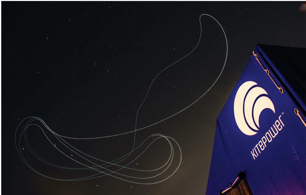
Photographic visualization of a pumping cycle during night operation on 11 October 2018 by tracing a marker light on the kite from the ground station (right) using long-term exposure (courtesy of Kitepower B.V.).
