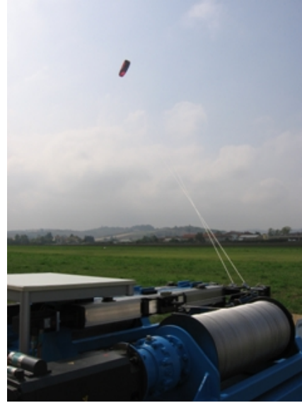
Fig. 4. Kite Steering Unit (KSU) small-scale prototype operating near Torino, Italy.
