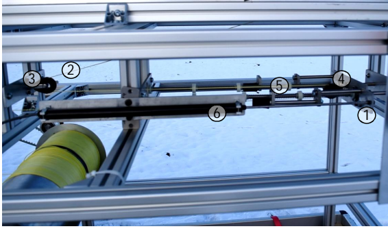
Fig. 4. Picture of the mass-spring system. The tether 2. passes through a stand-up pulley 4., attached to a mobile plate 1. which can move on steel shafts, each one supporting four springs in series, 5.. A linear potentiometer 6. is linked to the mobile plate and measures its displacement, i.e. the spring compression. One of the fixed stand-up pulleys 3. used to re-direct the aircraft tether is also shown.
