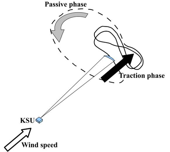
Fig. 3. Sketch of a KE-yoyo cycle: traction (solid) and passive (dashed) phases.
