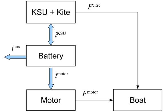
Fig. 4. Conceptual scheme of the hybrid kite boat.
