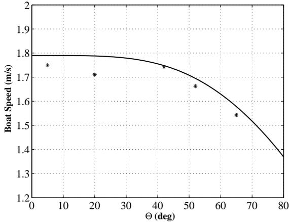
Fig. 10. Maximum achievable speed (solid line) as a function of angle  $\Theta$  between the boat and the wind directions, computed with the proposed method by considering the same conditions as those encountered during experiments in the KiteNav project, and comparison with experimental data (asterisks).
