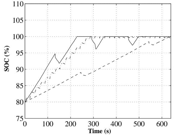
Fig. 15. Simulation results: battery state of charge obtained with  $\Theta = 0^\circ, 80^\circ, 180^\circ$ , dashed, solid and dash-dotted lines, respectively.
