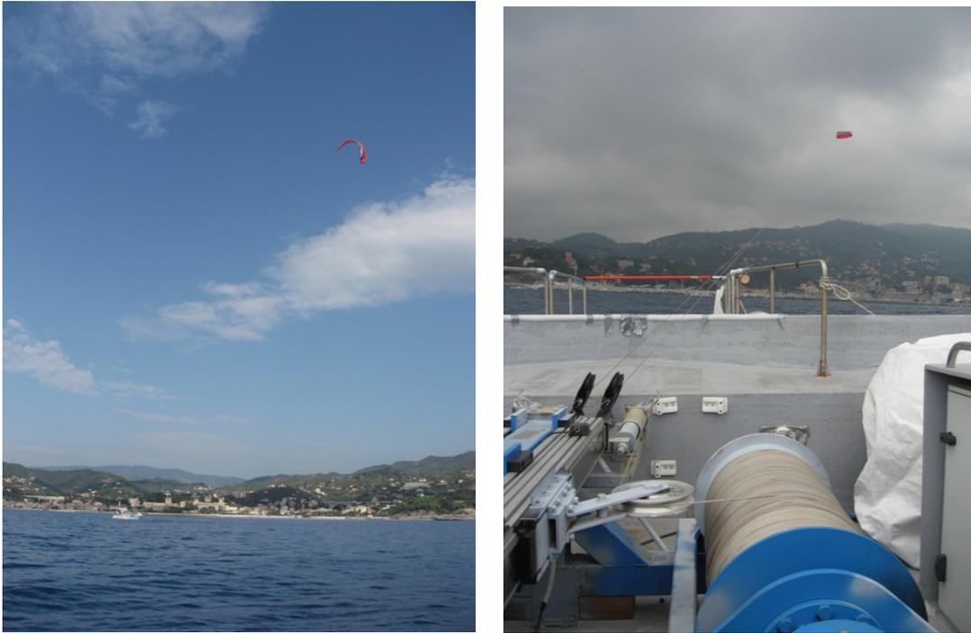
Fig. 2. KE-yoyo prototype installed on a boat and operating near Genoa, Italy.
