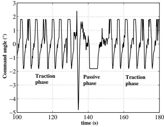
Fig. 11. Simulation results: example of the course of the input variable  $\psi(t)$  obtained with  $\Theta = 80^\circ$ , during traction and passive phases.
