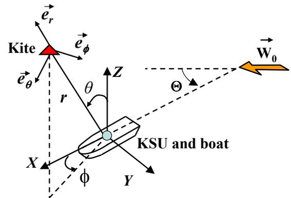
Fig. 5. Model diagram of the system.
