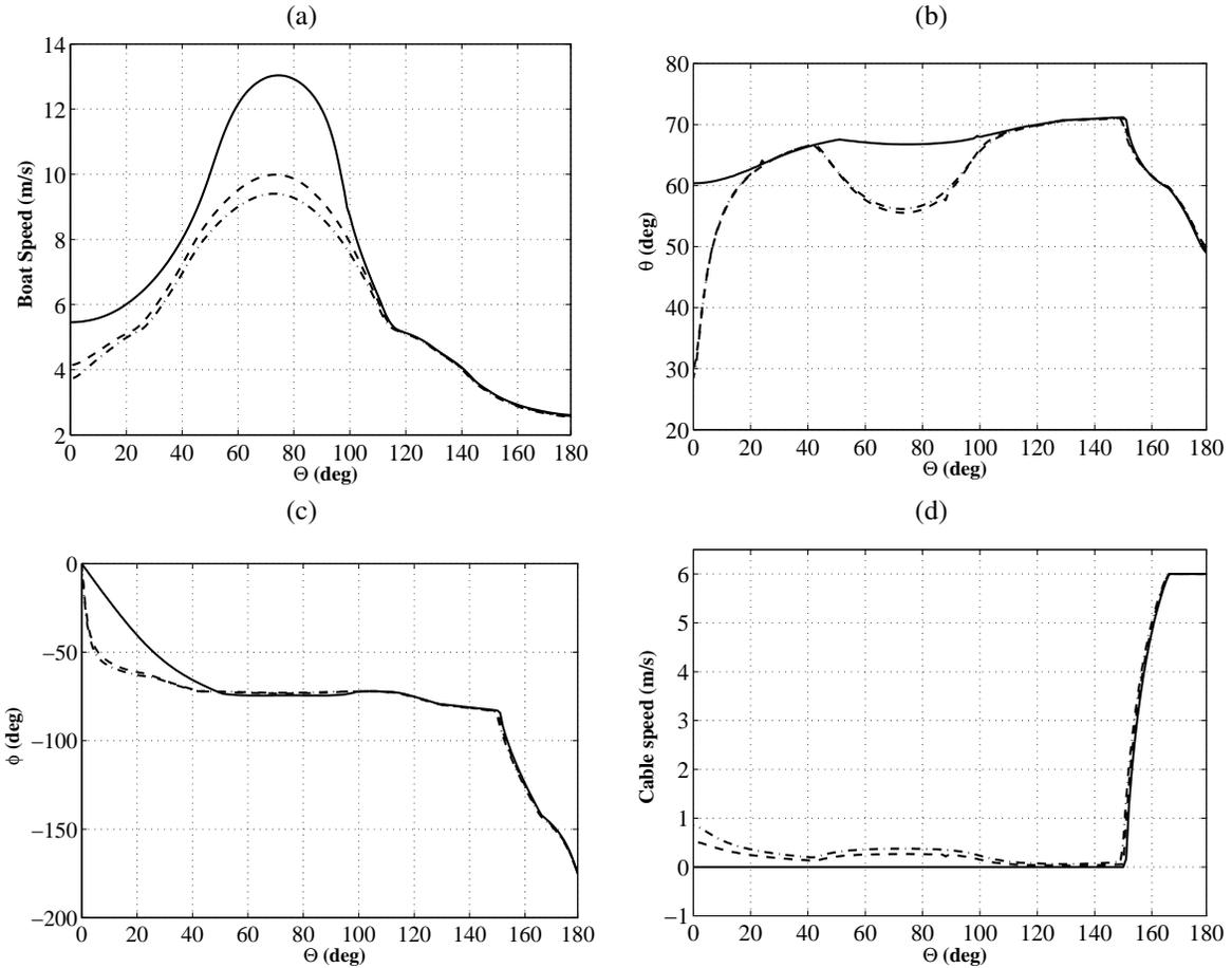
Fig. 9. Optimal operating conditions for a hybrid kite boat as a function of angle  $\Theta$  between the boat direction and the wind direction. Solid, dashed and dash dotted lines show results for value of  $P_{aux}^{elt}$  of, respectively, 0, 1 and 2 kW. (a) Maximum achievable speed  $v_{boat}^*$ , (b) angle  $\bar{\theta}^*$ , (c) angle  $\bar{\phi}^*$  and (d) line unrolling speed  $v_{ref}^{trac*}$
