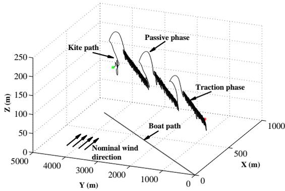
Fig. 12. Simulation results: boat and kite trajectories obtained with  $\Theta = 80^\circ$ . Boat starting position:  $(X, Y, Z) = (0, 0, 0)$ .
