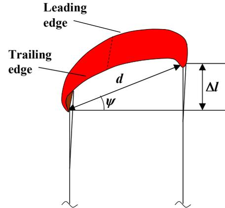
Fig. 7. Scheme of the control input  $\psi(t)$ .
