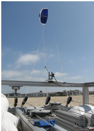
Fig. 4. Small-scale prototype built at the University of California, Santa Barbara, to study the control of tethered wings for airborne wind energy. The linear actuation system for the steering deviation, a load cell, the line angle sensor, the LEI kite and its lines are visible in the picture.
