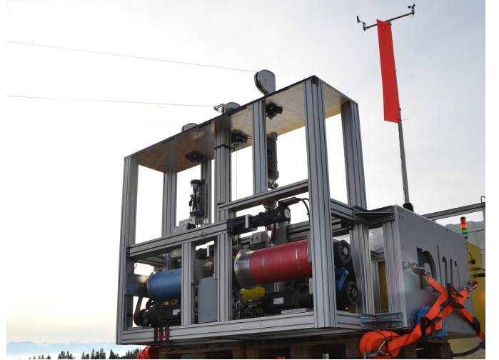
Fig. 1: Front view of the Swiss Kite Power prototype built at Fachhochschule Nordwestschweiz. The two steering lines, left (red) and right (blue), are wound around drums connected via a belt drive to motors mounted below the drums. The center line (yellow) wound around the main drum is behind the two other drums and is partly visible below the left steering line's drum. All three lines are guided separately via pulleys to the lead-out sheaves, visible at the top. On the lead-out sheave of the main line a line angle sensor is mounted. A wind sensor, mounted roughly 5 m above the ground, is visible in the background.
