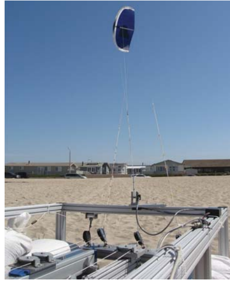
Fig. 1. Small-scale prototype built at the University of California, Santa Barbara, to study the control of tethered wings for airborne wind energy.
