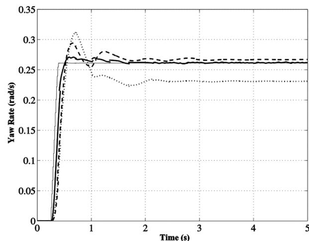
**Fig. 6** Results of the 50° handwheel step test when a blast of wind occurs at 1 s. Uncontrolled vehicle yaw rate (dotted line), reference yaw rate (thin solid line), and yaw rate obtained with the SMPC (solid line) and NMPC based on a physical model (dashed line) control laws
