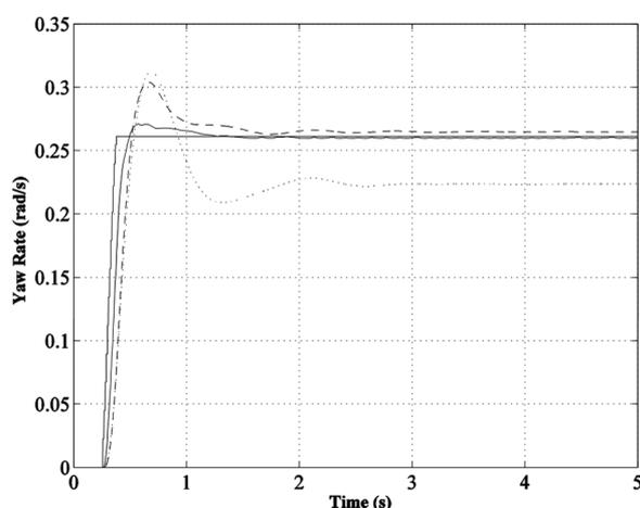
**Fig. 5** Results of the 50° handwheel step test with increased mass. Uncontrolled vehicle yaw rate (dotted line), reference yaw rate (thin solid line), and yaw rate obtained with the SMPC (solid line) and NMPC based on a physical model (dashed line) control laws
