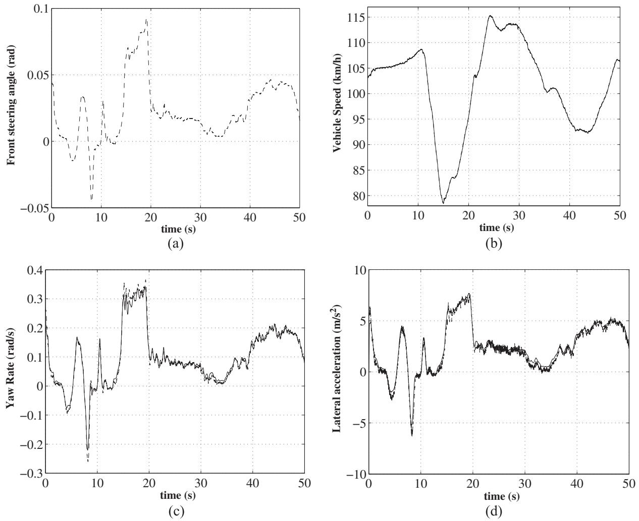
**Fig. 2** Comparison between real data (dashed line) and simulation results obtained with the 14-DOF model (solid line) during a track test: (a) front steering angle  $\delta$  (used as input for the 14-DOF model); (b) vehicle speed  $v$ ; (c) yaw rate  $\dot{\psi}$ ; (d) lateral acceleration  $a_y$
