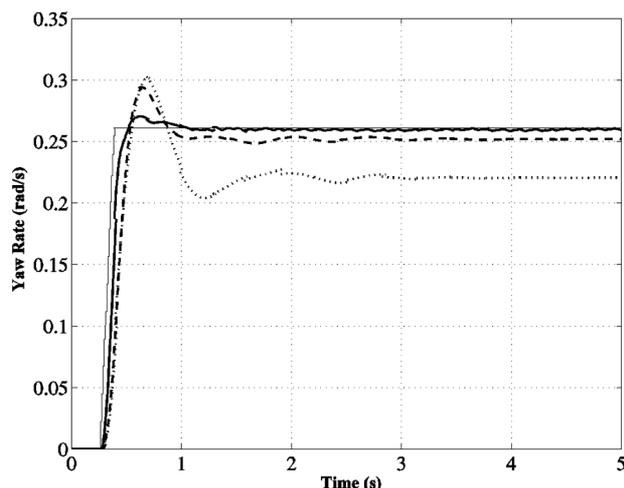
**Fig. 4** Results of the 50° handwheel step test with nominal parameters. Uncontrolled vehicle yaw rate (dotted line), reference yaw rate (thin solid line), and yaw rate obtained with the SMPC (solid line) and NMPC based on a physical model (dashed line) control laws
