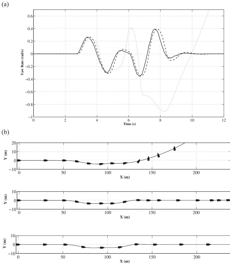
**Fig. 9** ISO double-lane-change test at 60 km/h on wet road: (a) yaw rate (dotted line, uncontrolled vehicle; solid line, vehicle controlled with SMPC controller; dashed line, vehicle controlled with NMPC controller); (b) vehicle trajectories (top, uncontrolled vehicle; middle, vehicle controlled with SMPC controller; bottom, vehicle controlled with NMPC controller)
