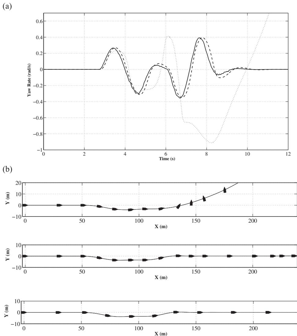
**Fig. 9** ISO double-lane-change test at 60 km/h on wet road: (a) yaw rate (dotted line, uncontrolled vehicle; solid line, vehicle controlled with SMPC controller; dashed line, vehicle controlled with NMPC controller); (b) vehicle trajectories (top, uncontrolled vehicle; middle, vehicle controlled with SMPC controller; bottom, vehicle controlled with NMPC controller)
