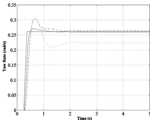
**Fig. 5** Results of the  $50^\circ$  handwheel step test with increased mass. Uncontrolled vehicle yaw rate (dotted line), reference yaw rate (thin solid line), and yaw rate obtained with the SMPC (solid line) and NMPC based on a physical model (dashed line) control laws
