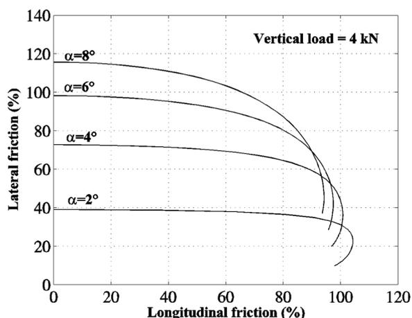
Fig. 1 Front tyre friction ellipses considered in the 14-DOF, with different values of lateral slip angle  $\alpha$  for a constant vertical load of 4 kN
