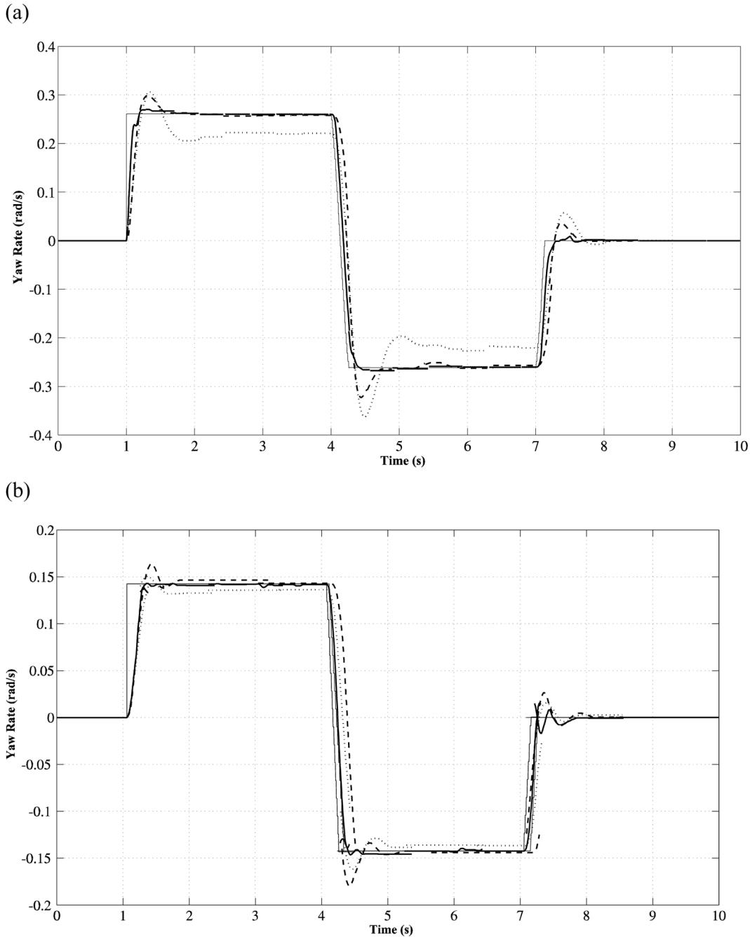
**Fig. 7** Steer reversal test: (a) 50° handwheel angle on dry road at 100 km/h; (b) 30° handwheel angle on wet road at 50 km/h. Uncontrolled vehicle yaw rate (dotted line), reference yaw rate (thin solid line), and yaw rate obtained with the SMPC (solid line) and NMPC based on a physical model (dashed line) control laws
