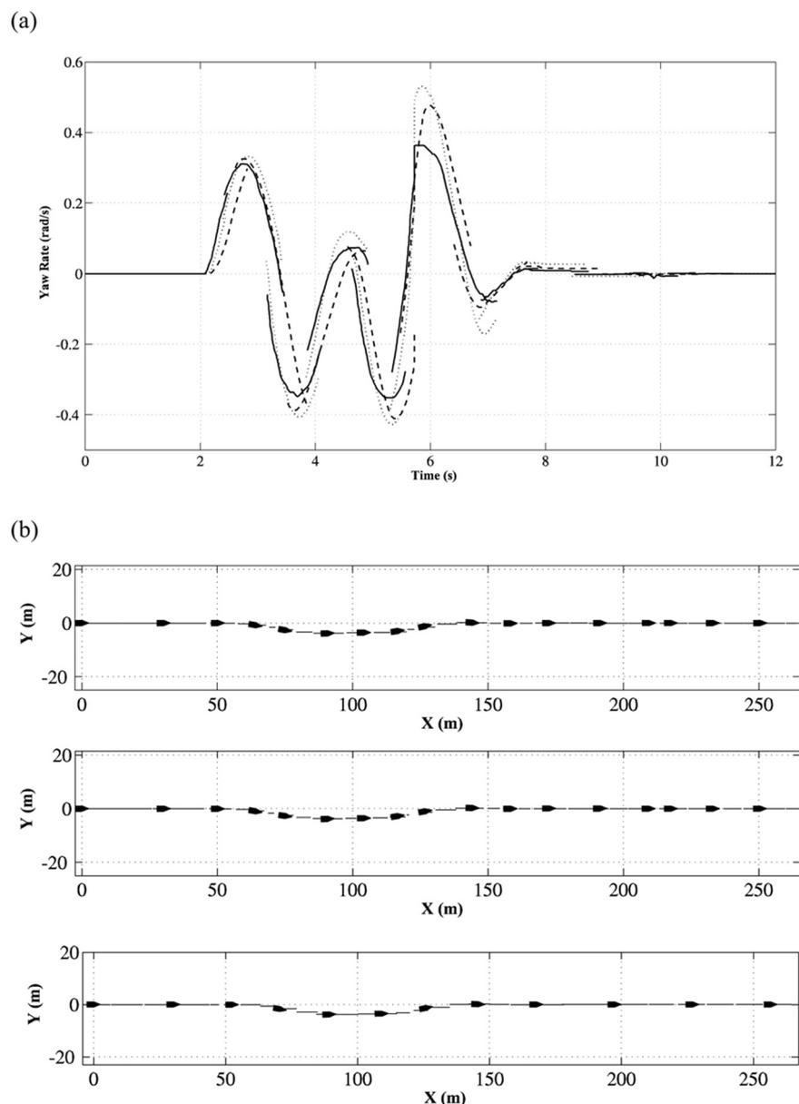
**Fig. 8** ISO double-lane-change test at 100 km/h on dry road: (a) yaw rate (dotted line, uncontrolled vehicle; solid line, vehicle controlled with SMPC controller; dashed line, vehicle controlled with NMPC controller); (b) vehicle trajectories (top, uncontrolled vehicle; middle, vehicle controlled with SMPC controller; bottom, vehicle controlled with NMPC controller)
