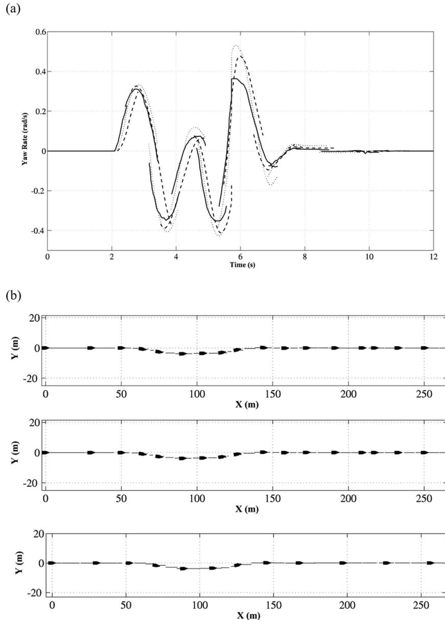
**Fig. 8** ISO double-lane-change test at 100 km/h on dry road: (a) yaw rate (dotted line, uncontrolled vehicle; solid line, vehicle controlled with SMPC controller; dashed line, vehicle controlled with NMPC controller); (b) vehicle trajectories (top, uncontrolled vehicle; middle, vehicle controlled with SMPC controller; bottom, vehicle controlled with NMPC controller)
