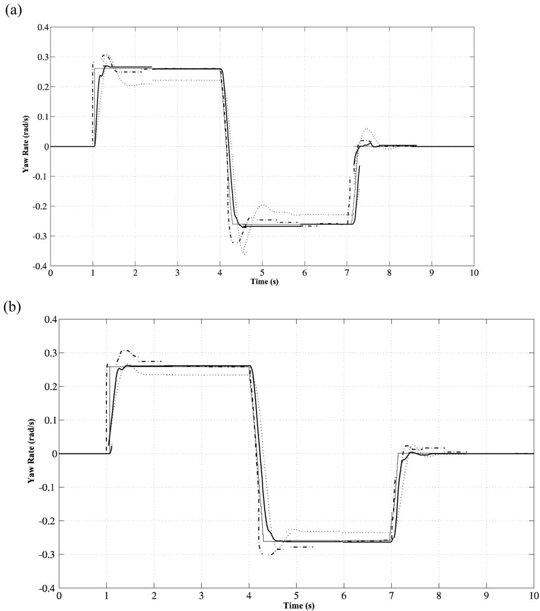
**Fig. 10** 50° steer reversal test performed: (a) at 100 km/h on dry road; (b) at 60 km/h on wet road. Uncontrolled vehicle yaw rate (dotted line), reference yaw rate (thin solid line), and yaw rate obtained with the SMPC (solid line) and IMC (dash-dotted line) control laws
