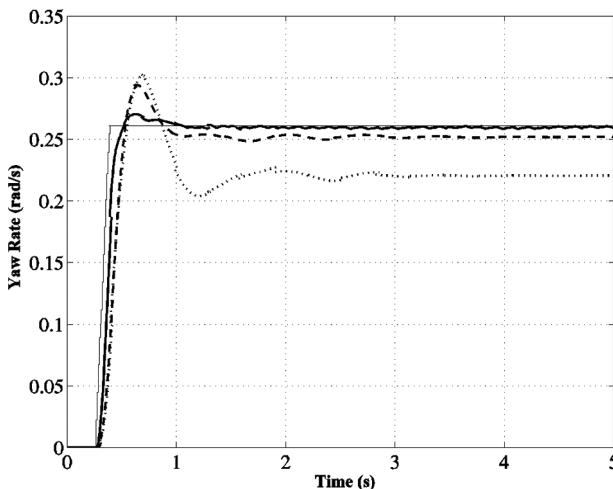
**Fig. 4** Results of the  $50^\circ$  handwheel step test with nominal parameters. Uncontrolled vehicle yaw rate (dotted line), reference yaw rate (thin solid line), and yaw rate obtained with the SMPC (solid line) and NMPC based on a physical model (dashed line) control laws
