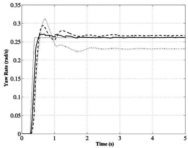
**Fig. 6** Results of the  $50^\circ$  handwheel step test when a blast of wind occurs at 1 s. Uncontrolled vehicle yaw rate (dotted line), reference yaw rate (thin solid line), and yaw rate obtained with the SMPC (solid line) and NMPC based on a physical model (dashed line) control laws
