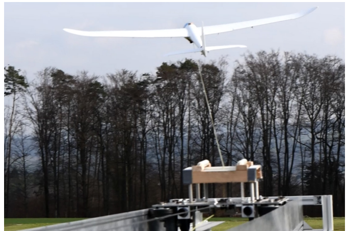
Fig. 10. Experimental case study: considered tethered aircraft during an autonomous take-off maneuver.
